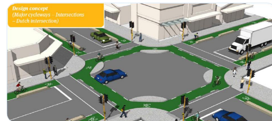
Figure 16: Key Infrastructure Elements of Protected Junction
