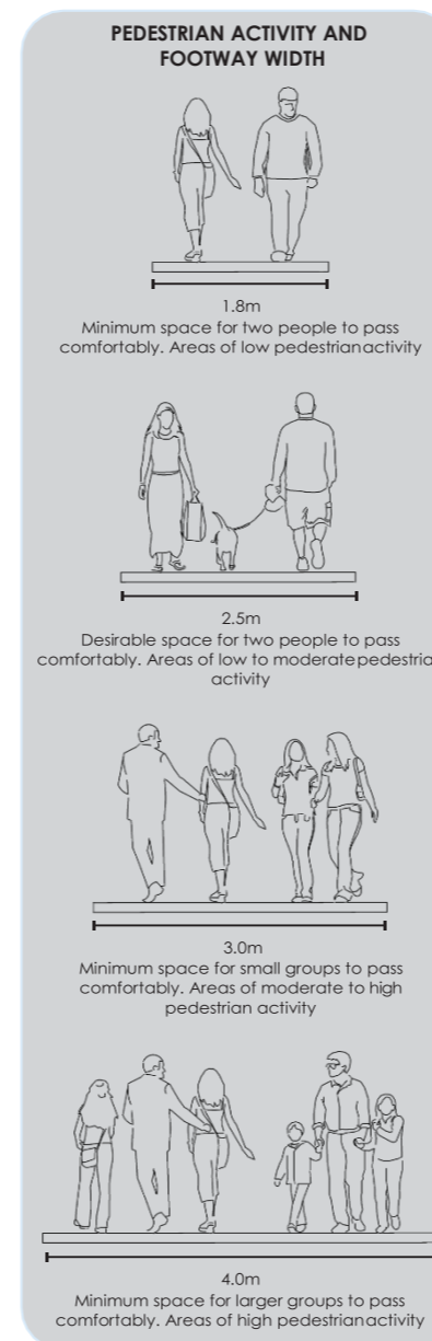
Figure 10: Extract from DMURS indicating appropriate footpath widths
